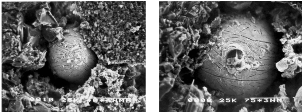
FIG. 11. Pore in concrete.
